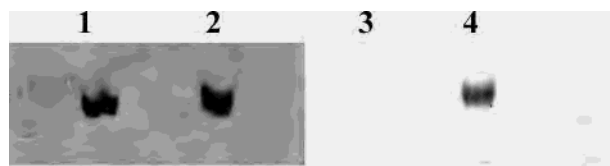
Figure 7. Native gel electrophoresis of L. innocua FLP on 5% PAGE. Coomassie stain of (1) unmineralized and (2) Co 3 O 4 mineralized L. innocua FLP cages, and 1-nitroso-2-naphthol stain of (3) unmineralized and (4) Co 3 O 4 mineralized L. innocua FLP cages.
